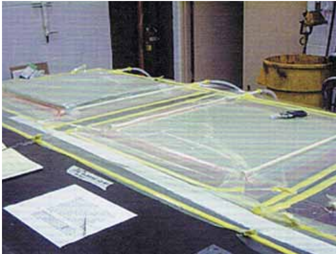
Fig. 1: 610 x 610 mm thin, flat plaque infusion set-up
