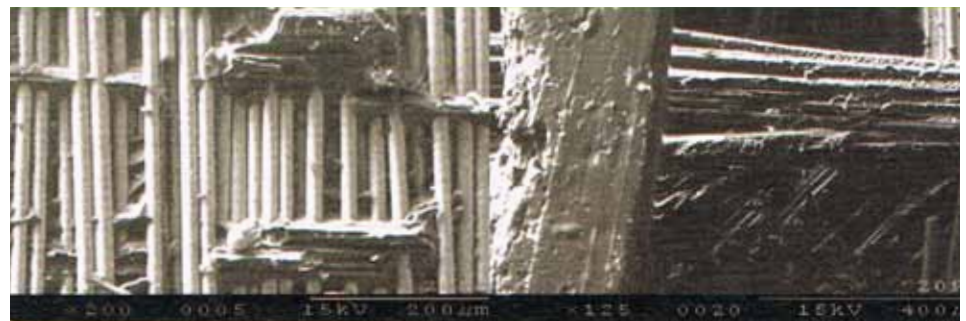
Fig. 10: SEM of fractured surface of epoxy/glass fibre composite
