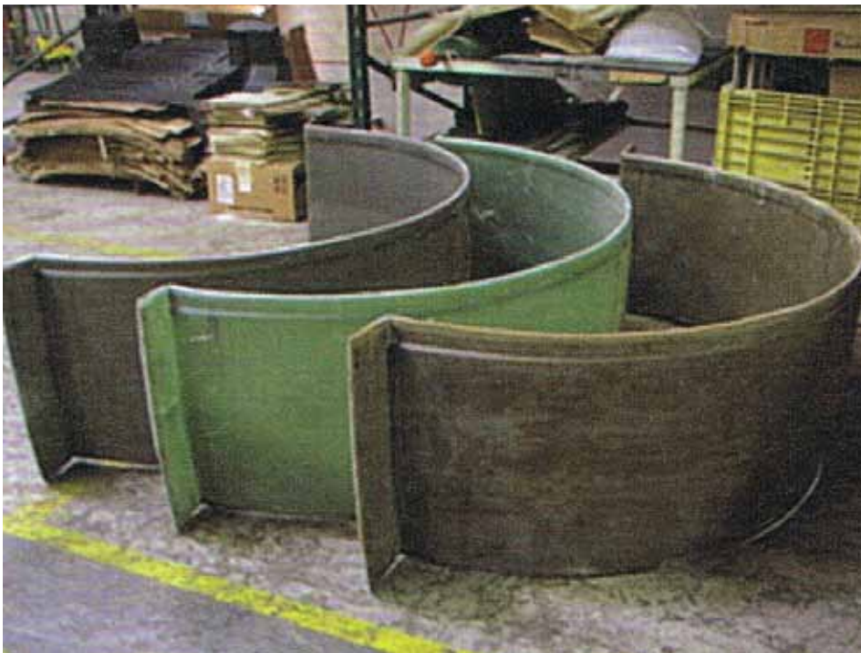
Fig. 3: Epoxy, vinyl ester and polyurethane root ring mouldings
